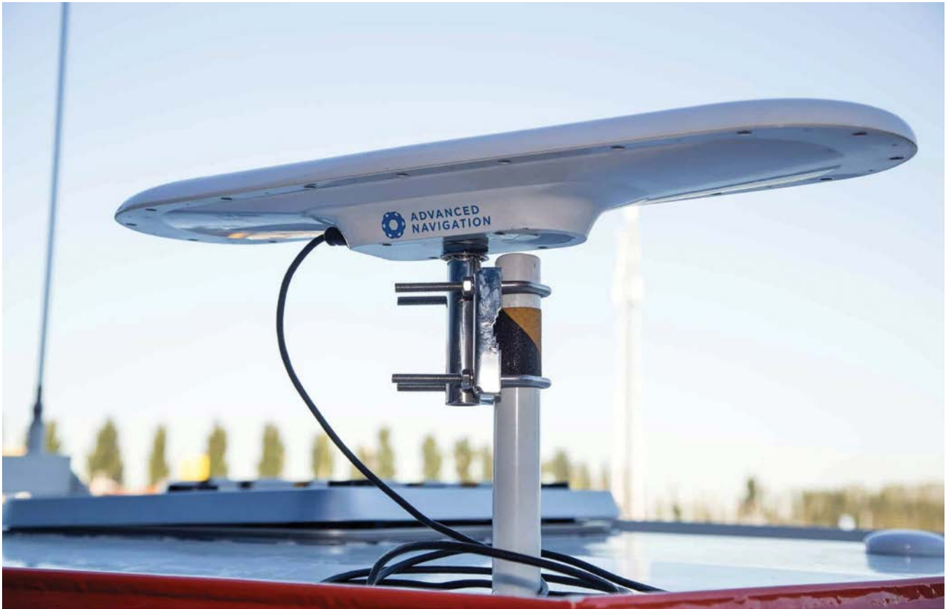
Advanced Navigation's GNSS compass installed on a vessel. Image: Advanced Navigation.
