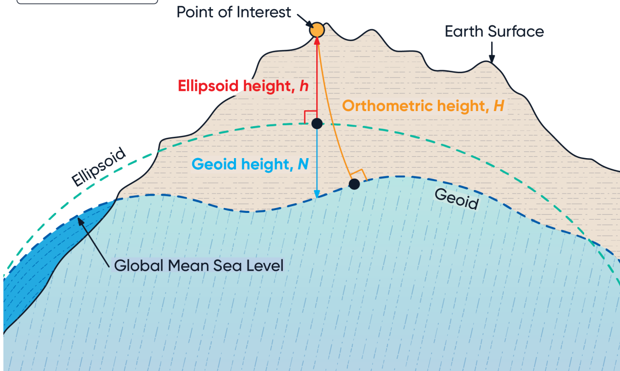
Illustration 6: Orthometric, ellipsoid and geoid height diagram
