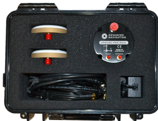
Illustration 9: Spatial FOG Dual Evaluation Kit contents
