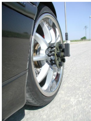
Illustration 23: Aftermarket wheel speed sensor
