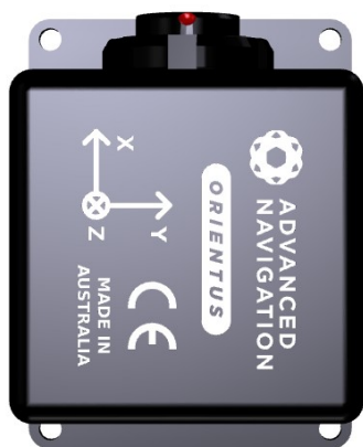
Illustration 1: Bird's eye view of Orientus showing axes marked on top
