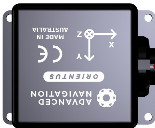
Illustration 8: Orientus after a heading change of 90 degrees
