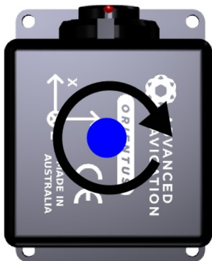
Illustration 7: Orientus with black arrow indicating positive direction of heading
