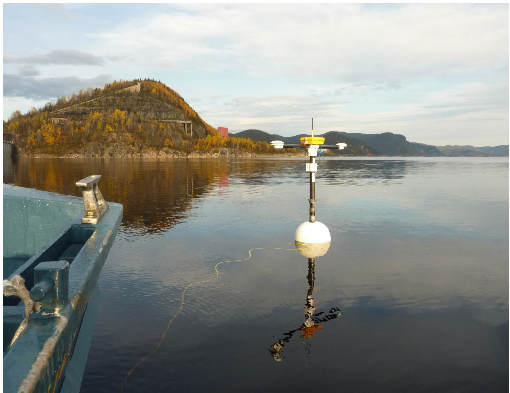
The RTKDuo USBL/RTK buoy used for a dam survey
