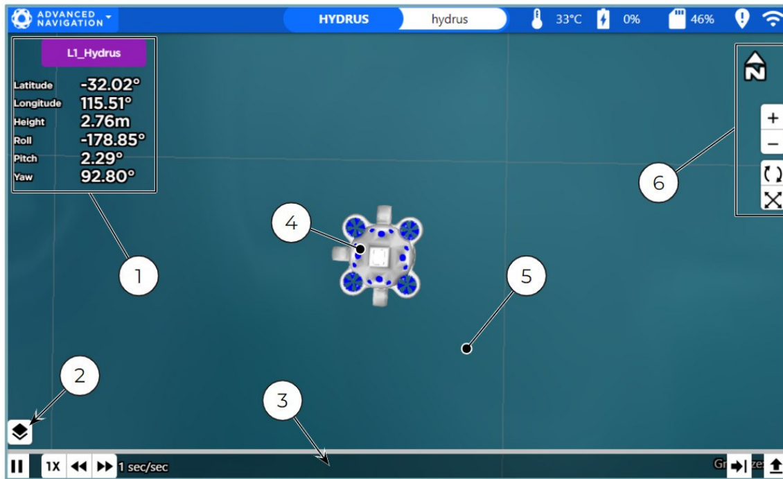
Figure 139: The Log Viewer page and its session playback pane is accessed by via Main Menu → View → Log Viewer .
