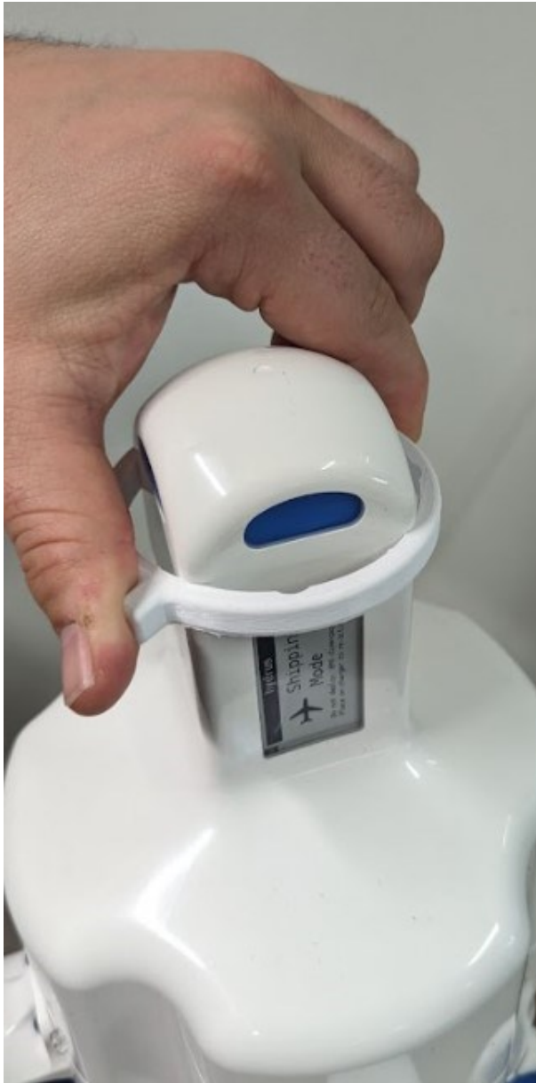
Figure 98: Test Clip Locking In
